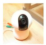
They typically feature two motors to rotate and tilt, sometimes a speaker and a microphone for two-way audio communication.
